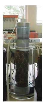
FIGURE 1. Configuration of the reactors used to the sludge samples inoculation. (1) reactor, (2) heated bath, (3) electric heater, (4) gases output, support medium.
