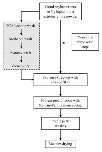
**Figure 1** - Schematic outline of the protocol presented here. The modifications performed on the original phenol/SDS method (Wang *et al.*, 2006) are shown in the dashed frames with a gray background.
