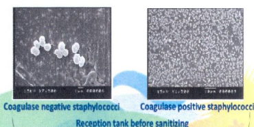
Figure 3A - Micrography of adhered cells of isolated strains on the surface of stainless steel AISI 304.
