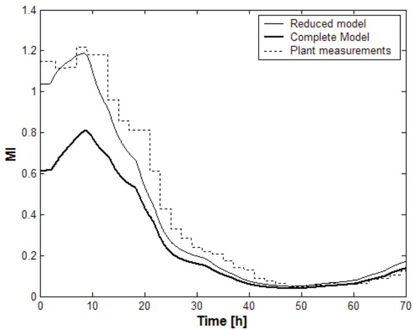
FIGURE 2.7 The plant measured melt index (MI) and the model simulated melt indexes.
