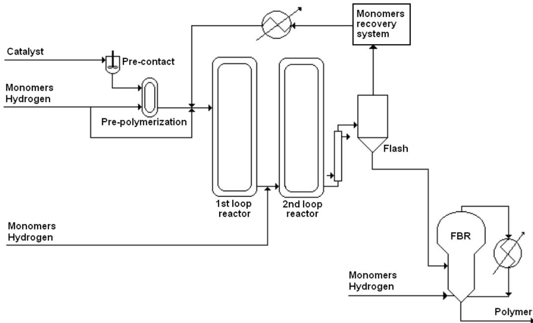
**FIGURE 2.3** SPHERIPOL process.
