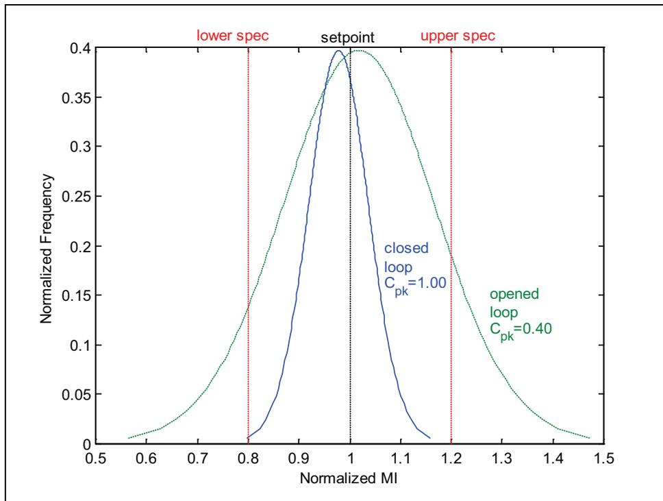
**FIGURE 2.13** Distribution curves for the opened loop and the closed loop.
