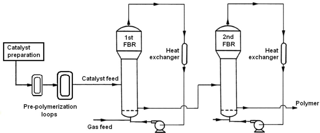
**FIGURE 2.2** SPHERILENE process.
