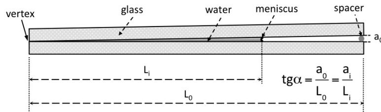
Fig. 1. Sketch of the dihedral tensiometer with a dihedral angle  $\alpha$ .
