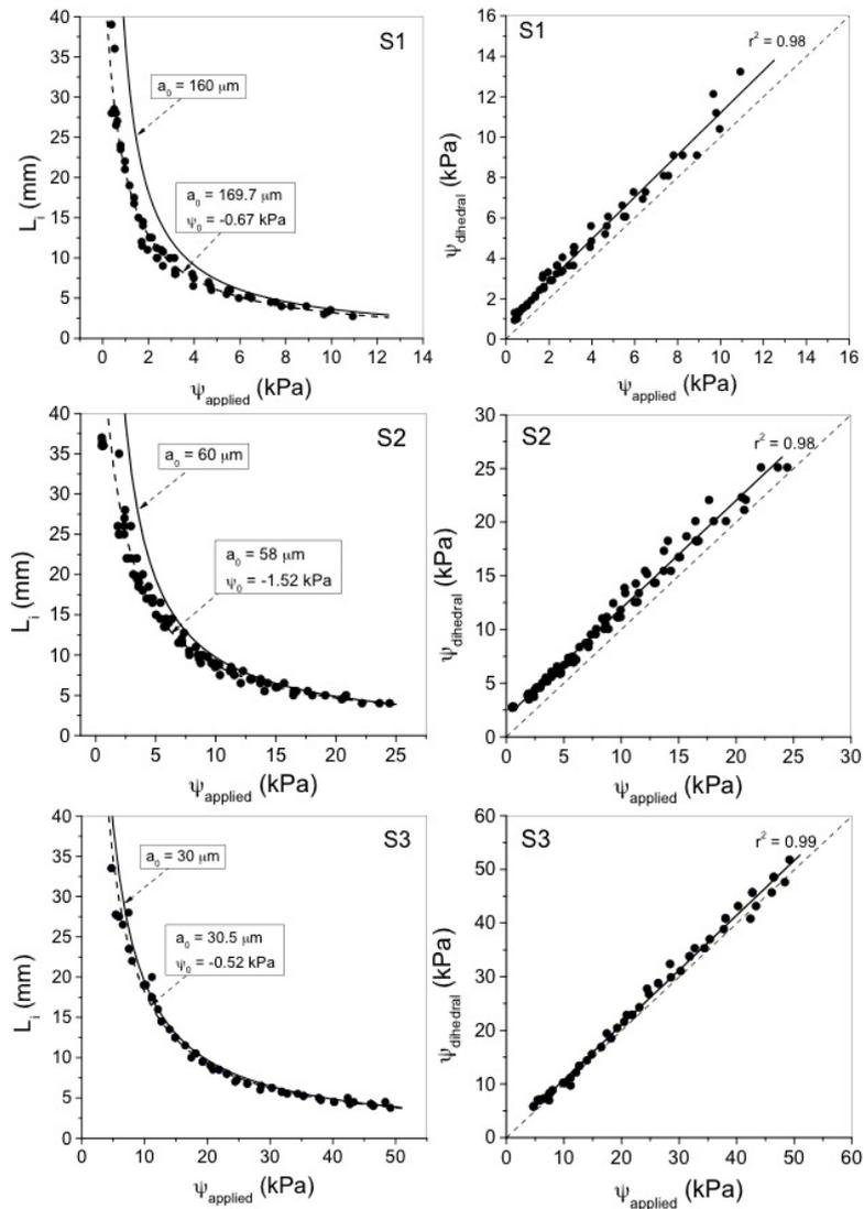
Fig. 5. Measured distance from vertex to meniscus ( $L_i$ ) as function of the applied suctions ( $\psi_{applied}$ ) (graphs on the left side) and comparison of  $\psi_{applied}$  and measured matric potential with the dihedral tensiometer ( $\psi_{dihedral}$ ) (right side), for S1, S2 and S3.
