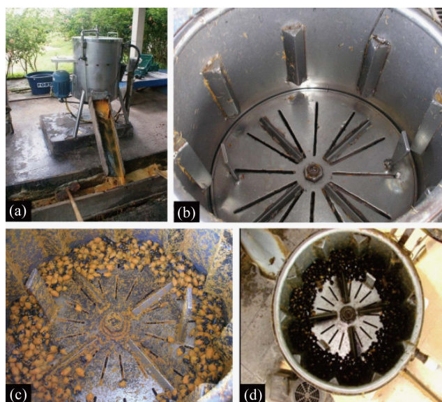
Figure 1. Mechanical depulper on the commercial production of oil palm seeds. (a) Front view; (b) Top view of the turntable; (c) Fruits in the depulper process; (d) Newly depulped fruit.
