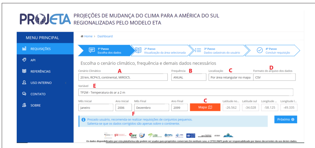
Figure 5: First step of the Web request - the user chooses of the request data in the PROJETA homepage: he must select the climatic scenario (A), the data frequency (B), the location (in this example a rectangular area) (C), the output file format for the requisition data (D), the climatic variable (E) and the initial and final data period (F) for the request.
