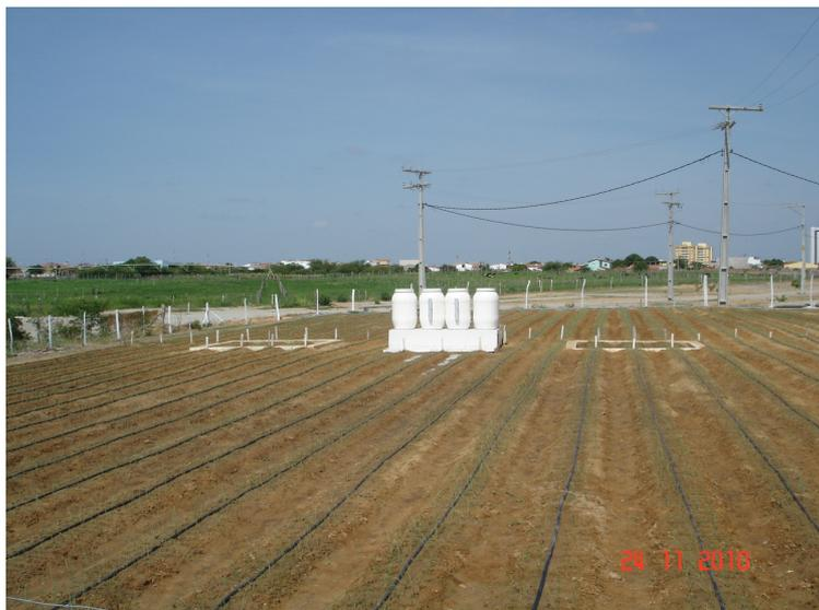
**Figura 1.** Área experimental contendo estrutura de evapotranspirômetros.(Experimental area with structure of evapotranspirometers). G. M. Oliveira, UNEB/DTCS, 2010.
